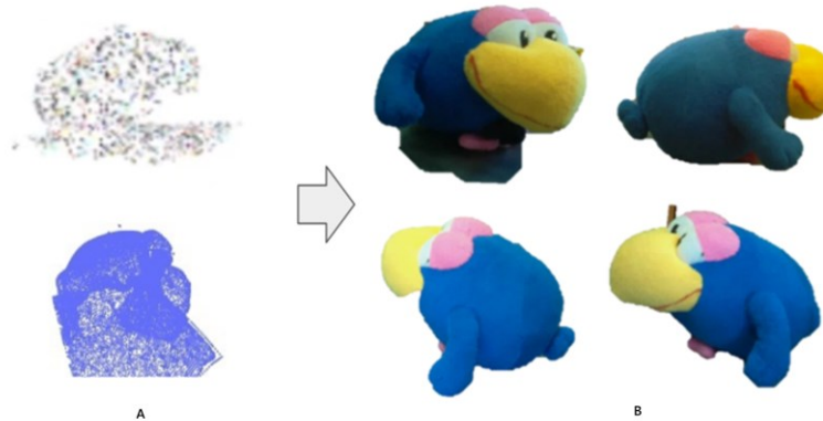
Figure 17. 3D object transformation. A. - Point clouds of the object (3D model), B. - Single images of the object from different angles.
